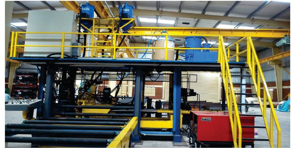
PEB BEAM WELDING SYSTEM
