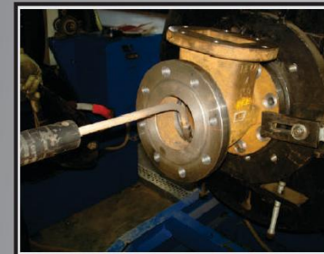
MECHANIZED SEAT RING SEAL WELDING SYSTEM
