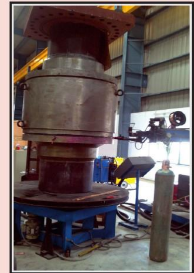
BALL VALVE ROOT TIG WELDING SYSTEM
