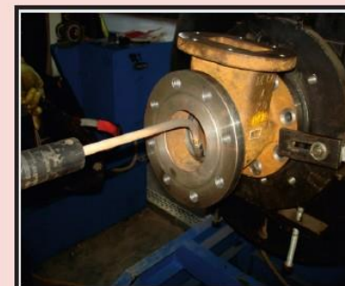
MECHANIZED SEAT RING SEAL WELDING SYSTEM
