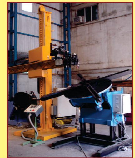
COLUMN & BOOM MANIPULATOR FOR SS BELLOWS WELDING
