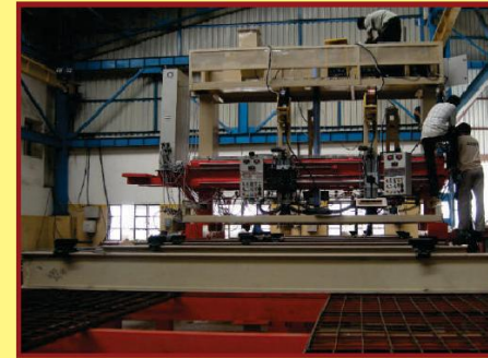
PANEL WELDING SYSTEM FOR BOILER MANUFACTURING
