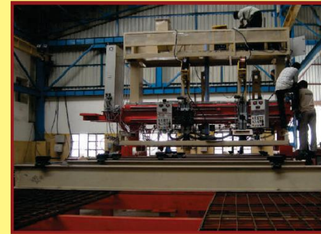
PANEL WELDING SYSTEM FOR BOILER MANUFACTURING
