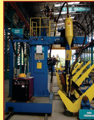
HEAVY BEAM WELDING AUTOMANTION
